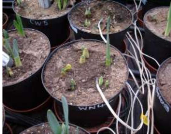
Thermocouples measuring soil at bulb depth within pots
