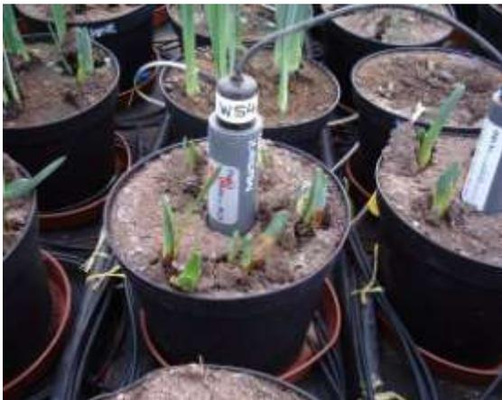
A Delta-T theta probe measuring soil moisture
